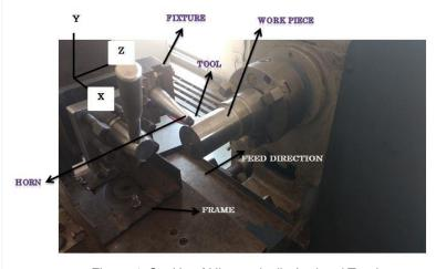
Figure 4: Set Up of Ultrasonically Assisted Turning
