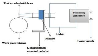
Figure 2: Schematic of Ultrasonically Assisted Turning
