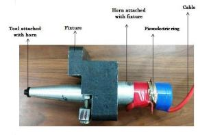
Figure 3: Tool and Horn Attachment
