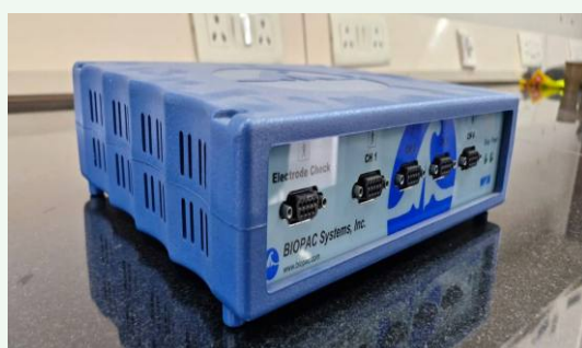
Data Acquisition System
