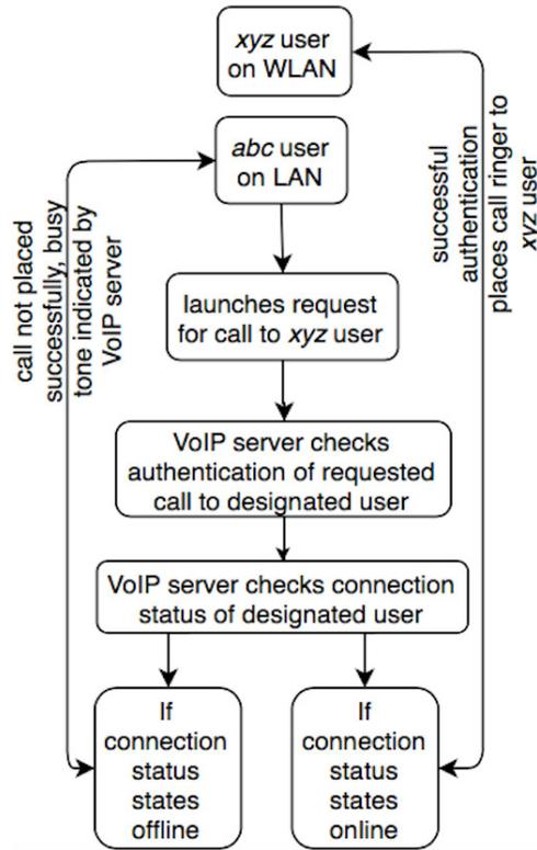
Fig. 7. Flowchart of call request from user *abc* to user *xyz* in module.
