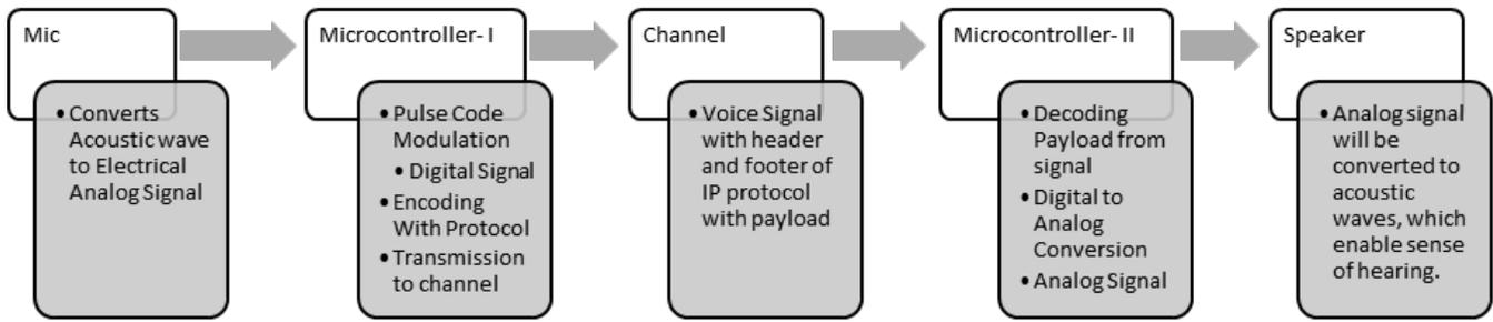
Fig. 1. Block Diagram of a basic VoIP system.
