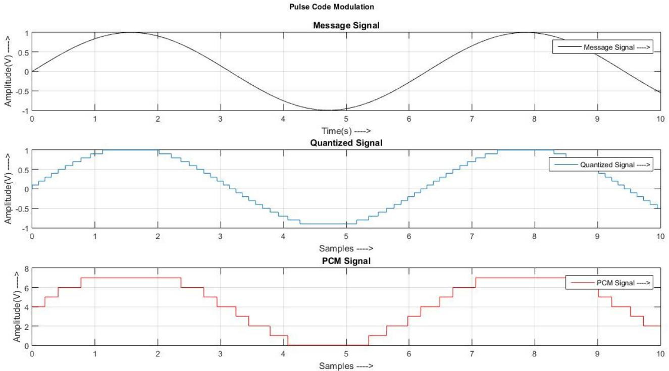
Fig. 3. Pulse code modulated sine wave with 256 quantization levels.
