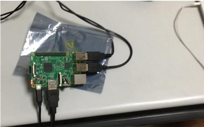
Fig. 4. RPi server on institutional WiFi in lab 1, powered by a standard mini-USB charger pin, with HDMI monitor & USB keyboard and mouse.
